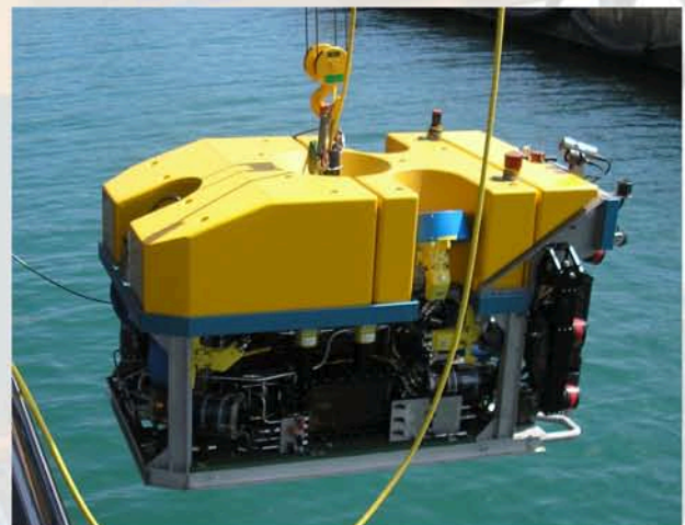
Larger 3000m DOER System being deployed
