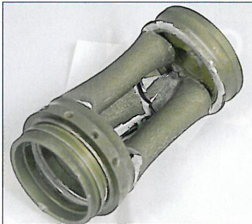
*(Above) A new pressure housing design was intentionally taken to crush depth to confirm the expected failure mechanism.*
