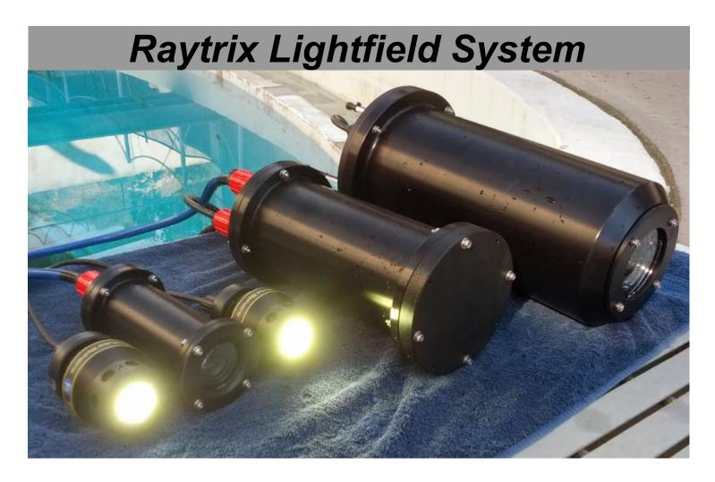
Compact, battery-powered, datalogging system for Raytrix lightfield camera
