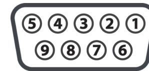
Figure 3-8: DB9 female socket numbering
