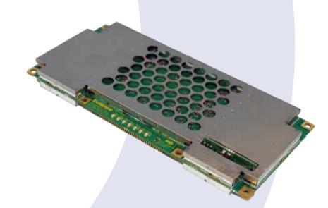
Develop sophisticated machine control and navigation solutions in a world full of complex dynamic environments. The Vector  $^{\mathbb{M}}$  H320 $^{\mathbb{M}}$  is our most advanced GNSS heading and positioning module available from Hemisphere GNSS.
