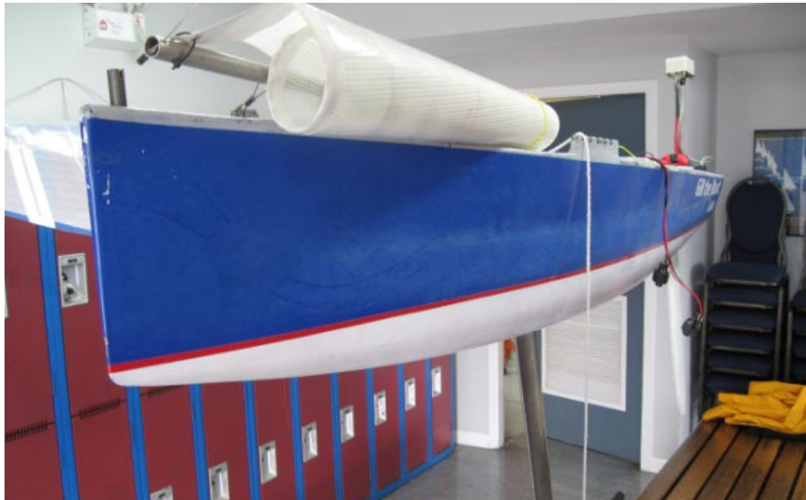
The most successful SailBot ever: "Gill the Boat" the U S Naval Academy's three time winner. Foil envy - note the beautiful CNC machined titanium keel foil!
