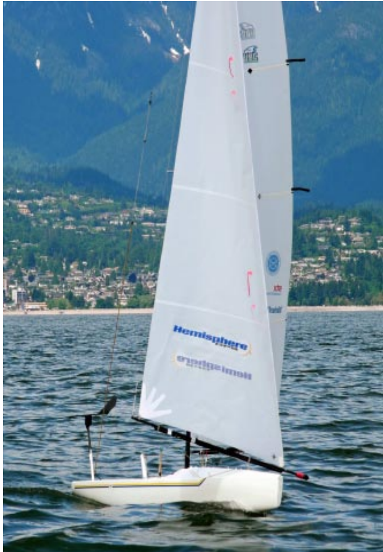
"Thunderbird 2012" sailing downwind under the biggest of her three rigs (code 0 rig - 12 1/2 feet - 0 to 8 knots true wind speed)
