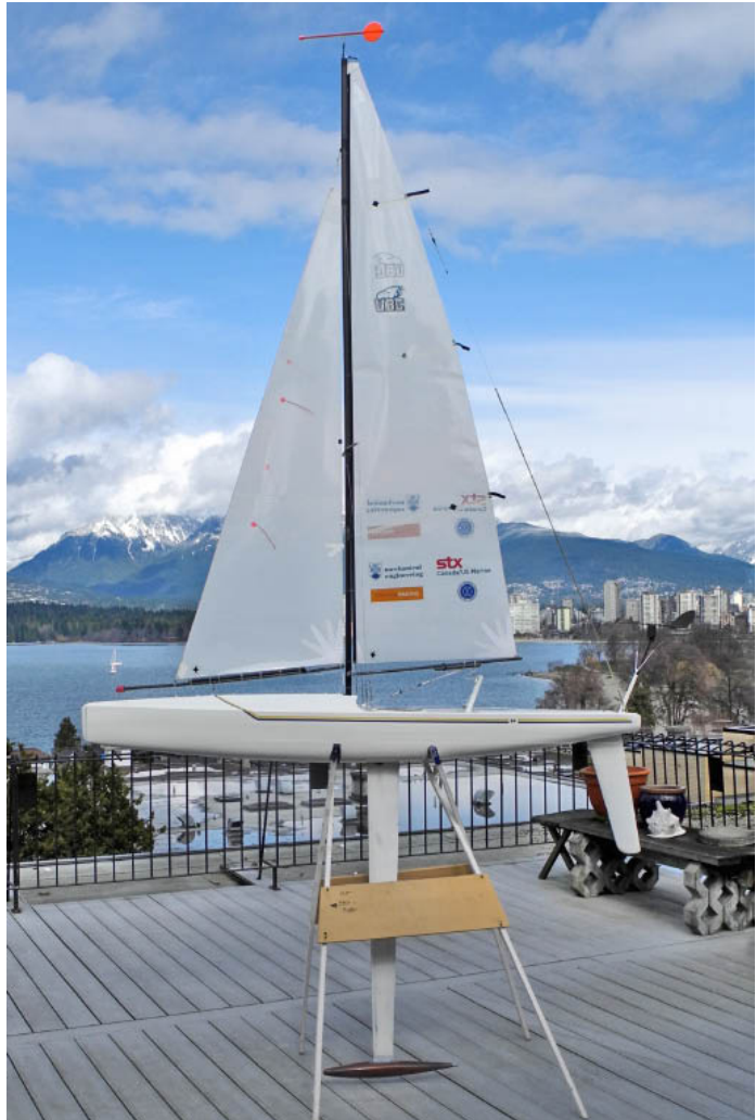
The smallest of the 3 rigs on Thunderbird 2012 – 8 ½ feet tall. The keel depth is 1.25M (50")
