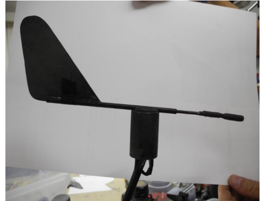
UBC's custom built carbon fiber wind sensor unit built around a Bourns optical encoder. Total weight with spar: 48 grams.
