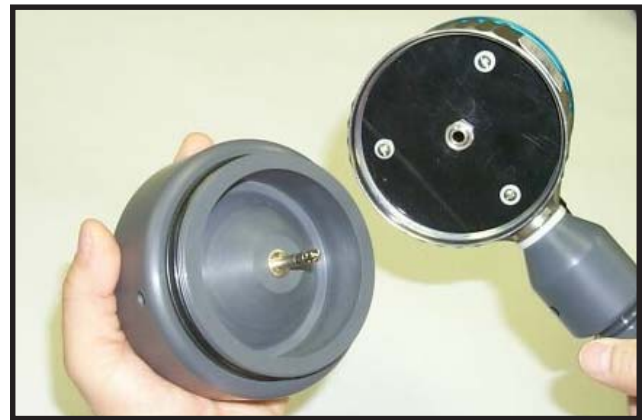
FIGURE 6. MATING HYDROPHONE WITH HYDROPHONE HOLDER
