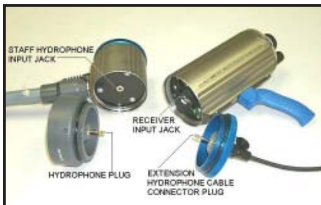
FIGURE 7. MATING EXTENSION HYDROPHONE CONNECTOR WITH A RECEIVER INPUT JACK.
