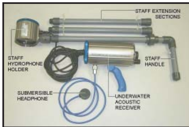
FIGURE 3. ACOUSTIC LOCATOR WITH SUBMERSIBLE HEADSET AND STAFF HYDROPHONE HOLDER (PRS MODE)
