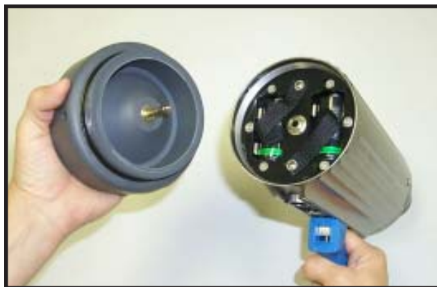
FIGURE 8. MATING HYDROPHONE WITH RECEIVER.
