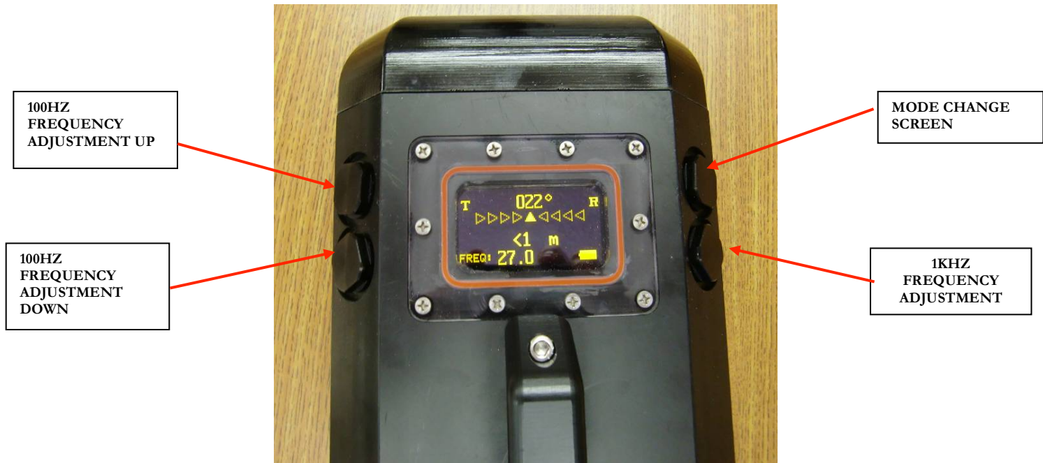
Figure 3-5 Display and Controls in Passive Mode
