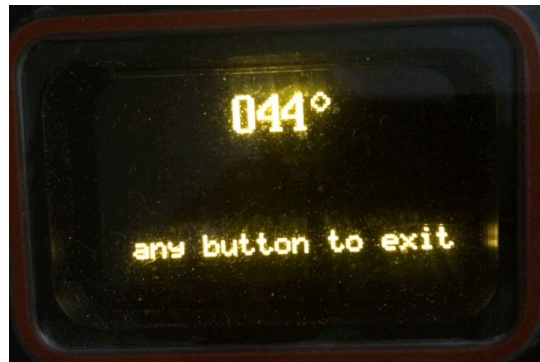
Figure 4-6 DTI-300 Compass Calibration is Complete
