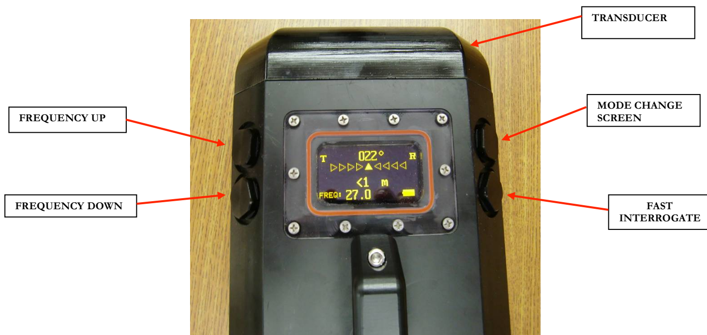
Figure 3-3 Display and Controls in Active Mode
