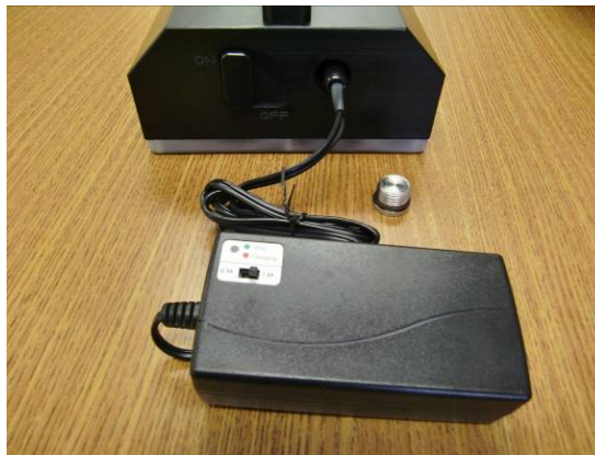
Figure 4-2 Charger Connected to DTI-300A
