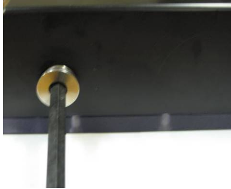
Figure 4-1 Charging Port Plug Removal
