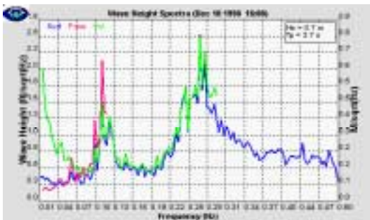
Figure 23. Amplitude spectrum of wave height derived from pressure (pink), ADCP velocities (green), and ADCP surface track (blue) for bottom-mounted instruments at 42m depth.
