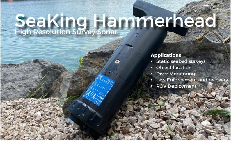
The SeaKing Hammerhead Survey Sonar utilises a wide transducer aperture, very fine mechanical step size and proven digital sonar technology to create high resolution imagery. Using the 675kHz frequency it is possible to obtain an overview of the site at up to 100m range and the 935kHz frequency allows a very high resolution scan at a range up to 40m.
