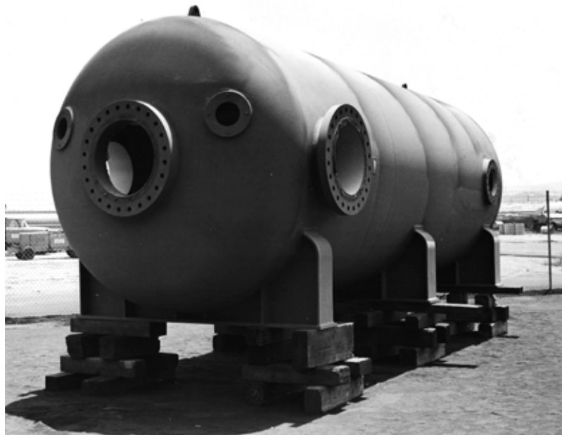
Saturation Systems' deck chambers. Courtesy Don Rodocker
