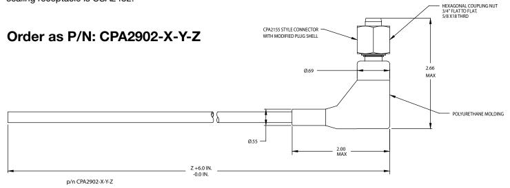
X = Form Code See Table 1 Y = Cable Code See Table 2 Z = Cable Length In Feet Use "0" If Ordering As Kit
