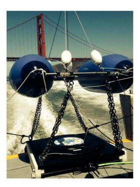
The **Falmouth Scientific Low Frequency Bubble Gun** is an acoustic seismic source that can be used independently or synchronized with other sources during off-shore, transition zone, and site surveys.
