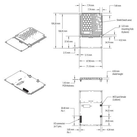
Figure 2-1: H200 mechanical layout
