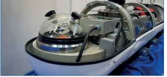
Instrument sphere in AUV
