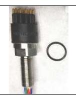
3. Screw the bulkhead connector into the adaptor finger-tight first and fully tighten it with a torque of 4 - 4,5 Nm.
