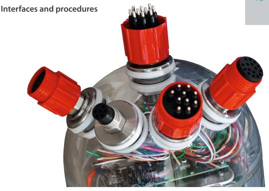
Pressure housings often require through-wall solutions for their unique combinations of connectors and sensors which moreover vary in diameter and length. For its VITROVEX® glass enclosures, Nautilus Marine Service has developed appropriate interfaces and specific manufacturing operations to this effect and supports its implementation.
