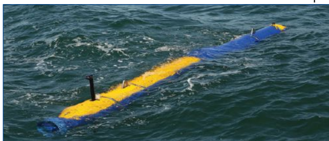
General Dynamics heavyweight, medium-class Bluefin-21 UUV and the Knifefish SMCM UUV. The Bluefin-21 modular construction and payload capacity provided the foundation for the Knifefish SMCM UUV program of record.
