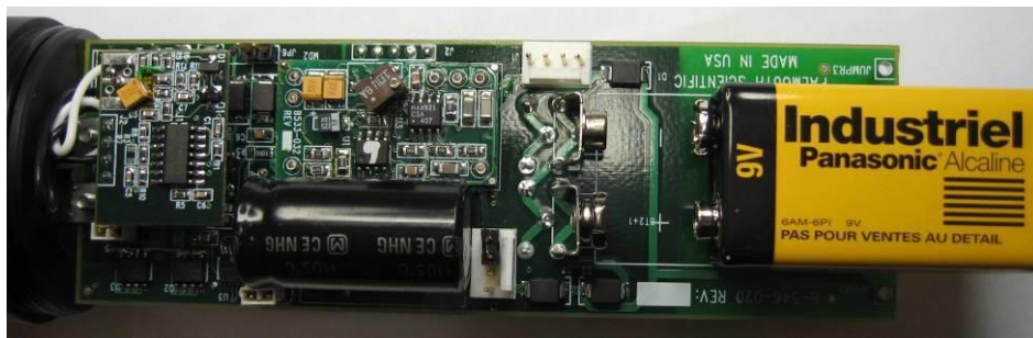
Figure 4-2 ATT-400 Battery Connections
