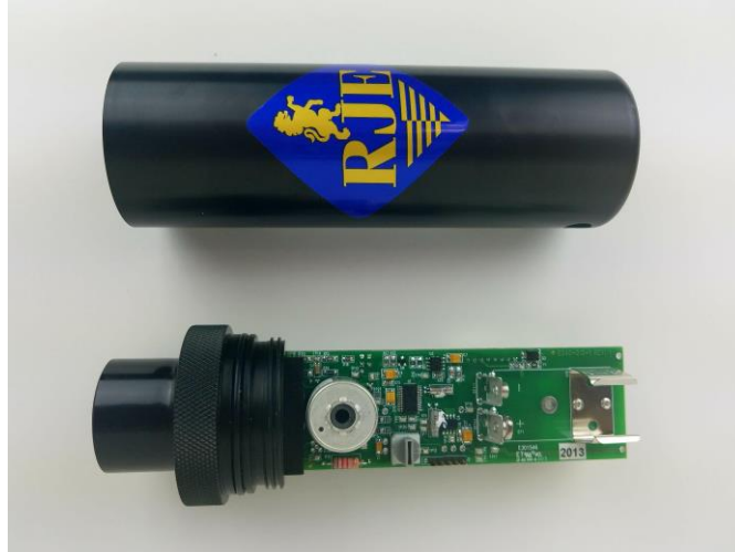
Figure 4-1 ATT-400 Disassembly
