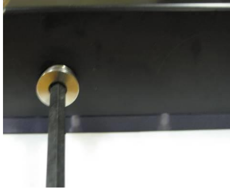
Figure 4-1 Removing the Port Plug
