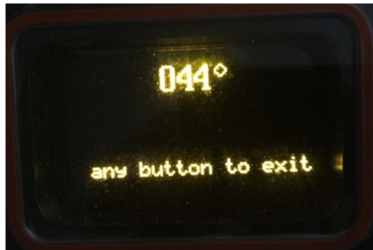
Figure 4-6 DTI-300 Compass Calibration is Complete
