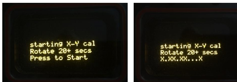
Figure 4-4 DTI-300A Hard Iron Compass Calibration X-Y Operation
