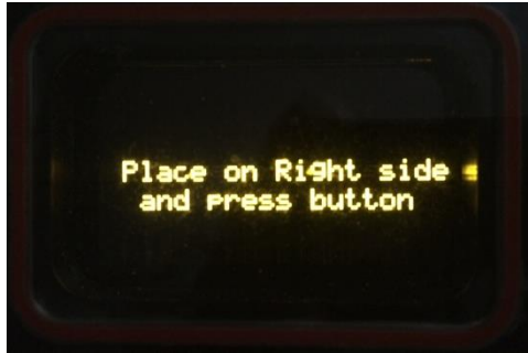
Figure 4-5 DTI-300A Hard Iron Compass Calibration Z Operation
