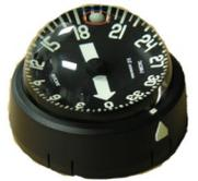
Illuminating the compass can be achieved by shining a bright light or UV light on the compass card for several minutes. This excites the luminous properties of the card and allows you to visually see the compass at night or in poor visibility conditions for up to eight hours. The longer you excite the card with light, the longer it glows underwater.
