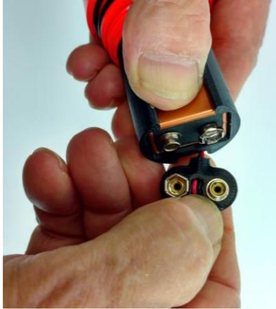
**Figure 4-1: Remove the Connector**
