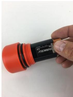
**Fig 4-3: Battery Installed and O-rings**
