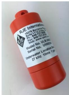
**Fig 4-4: Properly Assembled ULB-350**
