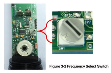
Set the switch position of SW1 to the position for the desired channel and/or frequency, using the table below for reference (Table 3-1):
