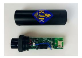
Figure 4-1 ULB-364 Disassembled
