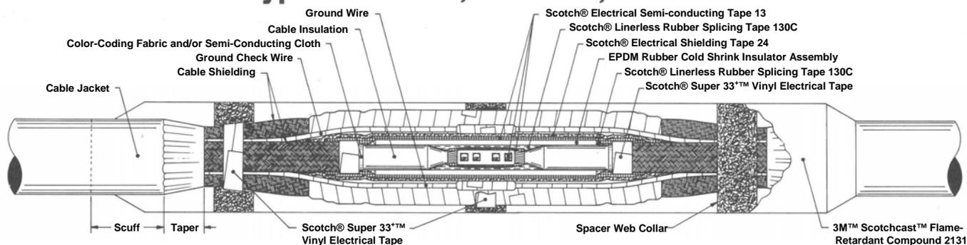
**NOTE:** On large 15 kV cables, additional Scotch® Tape 130C, Scotch® Tape 13 and Scotch® Tape 24 may be required.
