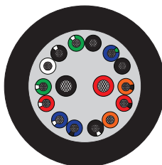
Type: P7TP22/2C18# 7 twisted pairs, 22 AWG 2 conductors, 18 AWG Nom. cable OD: 0.480", 12.20 mm
