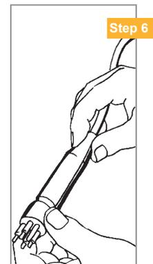
5. Select the appropriate polyurethane twin pack (e.g. 2131, 90 g for a single moulding) and mix the PUR material according to supplier instruction. Cut off the corner of the pack and squeeze the material into the boot as shown.
