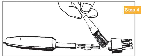
4. Degrease all moulding surfaces including cable jacket, conductors and brass body with acetone and allow to dry. Apply appropriate primer to brass body conductors, cable jacket and neoprene base of connector with a small brush and allow to dry (approx. 30 min. at 200°C). Do not touch primed surfaces after primer application.
