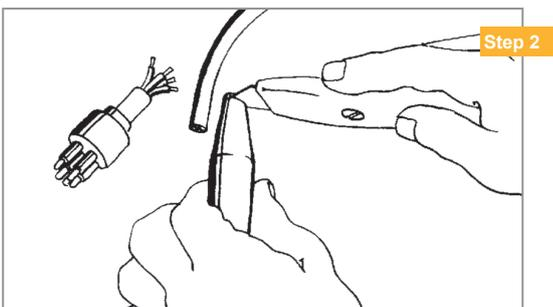
2. Cut pigtail wires on OM connector to approx. 2 cm from the brass body. Trim back tapered cable entry on boot until the cable is a snug fit (approx. 0.5 mm less than cable diameter).
