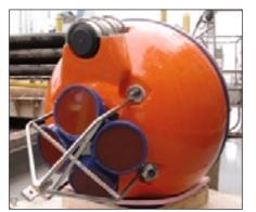
The one-metre diameter sphere with the embedded RDI ADCP and (at top) the Linkquest acoustic modem
