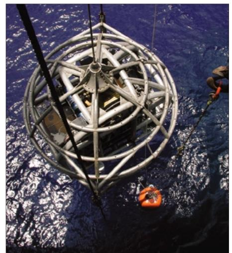
The Oceaneering ROV, with its tether management system, dives from *Deepwater Nautilus* to place the upward-looking current monitoring system on the seafloor in 1574m water depth in the Gulf of Mexico.
