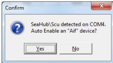
Click Yes on this pop up and the Channel Setup page will then automatically add and enable the main COM Port for the SeaHub.
