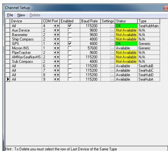
Once all the ports have been identified, the `Enabled` box can be checked for each port that is required.
