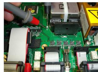
Both these fuses are 2A surface mount “Quick Acting” fuses. If either has blown the most likely cause is excessive current drain from an externally connected device (5V for USB peripherals is protected by over-current limiting circuitry to prevent damage) – review your power setup, requirements and jumper settings. However, it is recommended to contact *Tritech International Ltd* for further assistance.
