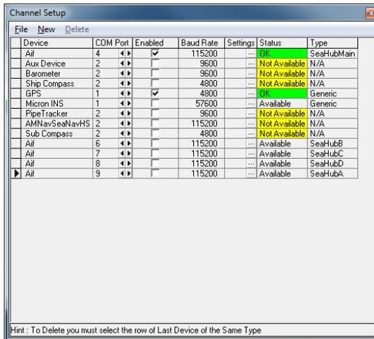
From the list of available AIF devices, identify the one that is linked to the SeaHub Port that you need to connect your device. Ensure that it, and the SeaHubMain port, are the only SeaHub Ports left enabled.
