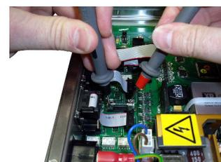
If the fuse has blown, use a screw-driver to carefully remove it from its holder (the body of the fuse is glass!), and replace with a “2A 250V 20x5mm Quick-Acting (F)” fuse
