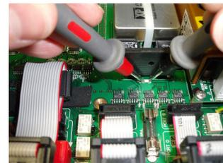
Use a continuity tester to determine if the fuse “F4” has blown – supplying the +5V supply.
