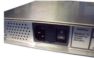
Open the fuse tray using a small, flat-bladed screwdriver. There are retention clips at the top and bottom of the tray and it is important not to force it too much in case they break.
