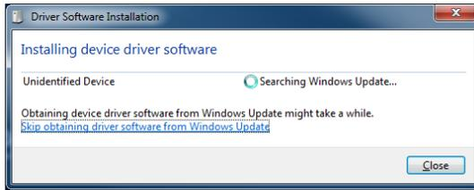
By default, Windows will try to load the latest drivers from the Windows Update service, but this is not required as all the appropriate drivers are installed along with Seanet Pro. Click on the Skip obtaining drivers from Windows Update link.
