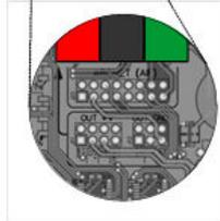
The PCB silk screen details the various connections possible using the headers.
