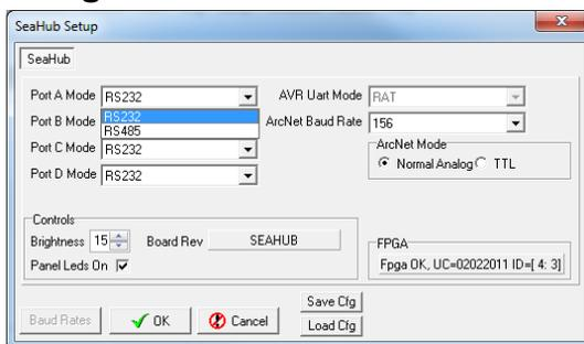
These drop down selection boxes change the communication protocol that the Port will operate on. For serial based communication protocols (RS232, RS485 and RS422) the Baud rates are controlled through the Channel Setup and not directly via the SeaHub.
