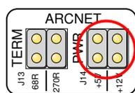
Using a 2.5mm jumper, Select either the +5V or +12V option from the J14 header
