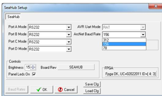
This drop down selection box changes the baud rate for ARCNET communications.
