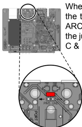
When operating Ports C and D in ARCNET Comms Mode, ensure that the top row pins of J19 and J22 are shorted together before connecting ARCNET Dual Head Profilers to Ports C & D. The diagram to the right shows the jumper position for this configuration which results in Pin 5 of DIN Ports C & D being linked together (and isolated from Comms Ground).
