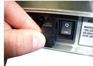
Both the top and bottom fuse are required for correct operation of the Rack mount SeaHub. As with the Desktop version, any replacement fuses should be “2A 250V 20x5mm Antisurge(T)”.
