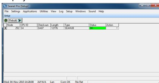
From the drop down menu at the top of the screen select `Utilities` then `Com Setup`.
