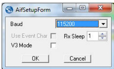
The default Baud rate for a SeaHub Port is 115200. This can be changed by using the drop down list.
