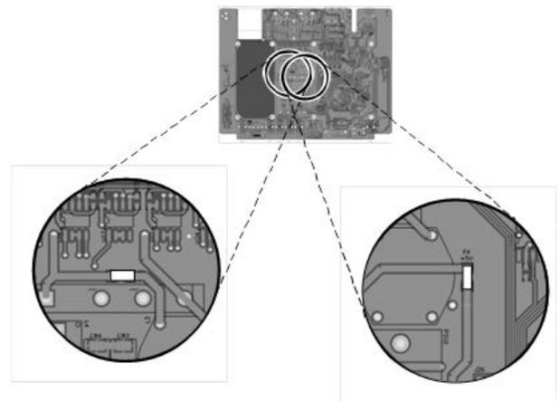
Use a continuity tester to determine if the fuse “F2” has blown – supplying the main PCB power from which both +12V and +5V is derived.
