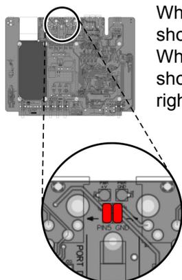
When operating Port C in RS-232 Comms Mode, ensure that J19 is shorted, as indicated by the left jumper position in the diagram to the right. When operating Port D in RS-232 Comms Mode, ensure that J22 is shorted, as indicated by the right jumper position in the diagram to the right.
