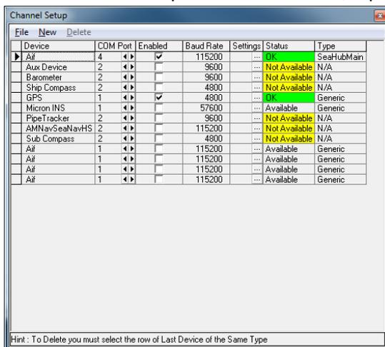
Once the addition AIF devices have been added, use the left and right arrows within the COM Port to identify the various ports on the SeaHub.
