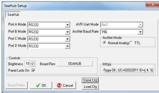
This Setup window enables the user to change the operation of each port of the SeaHub as well as modifying the baud rate for ARCNET communications
