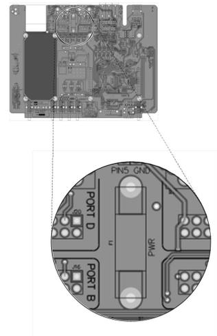
Use a continuity tester to determine if the fuse has blown. If the fuse has not blown contact *Tritech International Ltd* for further assistance.
