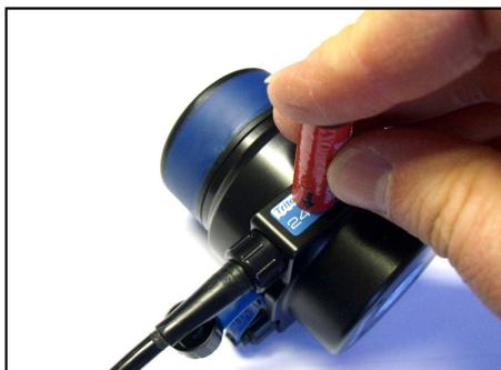
**Figure 5.2. Location of Reset Switch (activated by magnet)**
