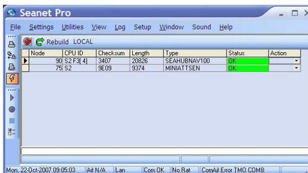
The SEAHUBNAV100 and MINIATTSEN device types should be visible in the Setup window. The MicronNav100 Hub must now be configured to communicate directly to the Transponder/Responder in order to carry out the conversion. In Seanet Setup click the Action column in the SEAHUBNAV100 row followed by Setup from the drop-down menu that appears to display the SeaHub Setup page. Set Port B to RS232.
