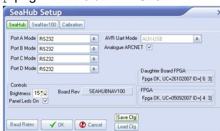
Confirm the settings and close the SeaHub Setup page. After a few seconds, the reprogramming of the unit will be complete and "Node 90, Prog Cfg Done" will be displayed in the status box. The SEAHUBNAV100 table entry will temporarily disappear from the list while the unit resets to activate the change.
