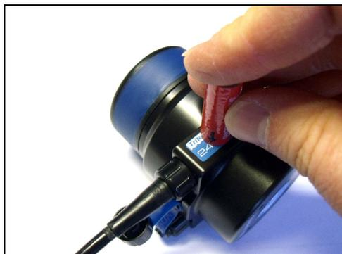
After a few seconds the unit should be visible in the Seaset Setup window (and displayed as MINIMODEM). If not try repositioning the magnet slightly and power-cycling again.
