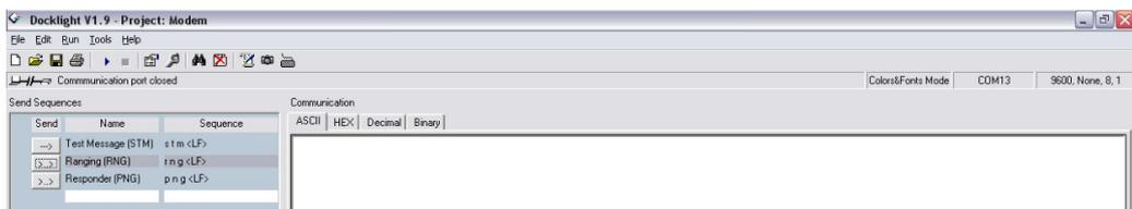
3. The COM port that the Micron Data Modem is attached to needs to be configured. Double click on the COM port number in the top right hand corner of the main window which will open the Project Settings dialog. Within this dialog select the appropriate COM port for the modem to be used. Ensure the baud rate is set to match the modem (9600 by default) and that the Send/Receive option is selected.
