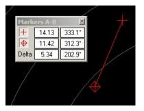
Adds a Markers A-B dialog to the screen where to markers can be selected/de-selected and moved using the mouse. When a marker is first selected it appears on the origin of the sonar scan and if it is subsequently de-selected it will lose any of its positional data. When both markers are selected a line is drawn between them and the relative distance and bearing between them is shown.
