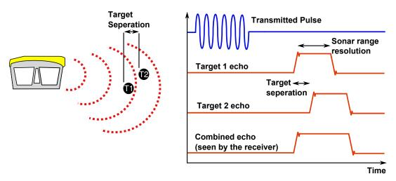
Using the example above, if two targets are less than 37.5mm apart then they cannot be distinguished from each other. The net effect is that the system displays a single large target, rather than multiple smaller targets.
