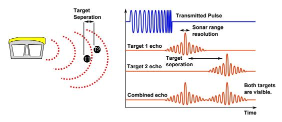
The response from the pattern-matching algorithms in the sonar means that the length of the acoustic pulse no longer affects the amplitude of the echo on the sonar display. Longer transmissions (and operating ranges) can be achieved without a loss in range resolution.
