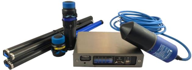
The system comprises a subsea Micron Modem or Battery Micron Modem, a surface USBL transducer with integral magnetic compass and pitch/roll sensors, a surface MicronNav 200 interface hub and bespoke operating software under control of a topside PC/laptop.
