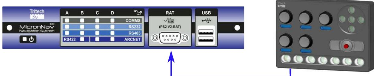
Power the MicronNav 100 and the Windows Hardware Wizard will auto-install the device from the pre-installed driver package.
