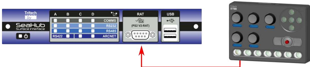
Power the SeaHub and the Windows Hardware Wizard will auto-install the device from the pre-installed driver package.
