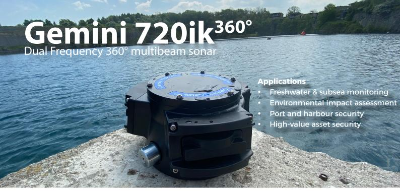
Using proven technology from the Tritech Gemini 720ik multibeam imaging sonar, the Gemini 720ik $^{360^{\circ}}$  is a fully integrated and cost-effective underwater monitoring system. With a 360° field-of-view, a large underwater environment can be monitored in real-time. Unlike mechanical scanning sonars, the Gemini 720ik $^{360^{\circ}}$  generates 1536 beams simultaneously, making it ideal for monitoring targets in motion.
