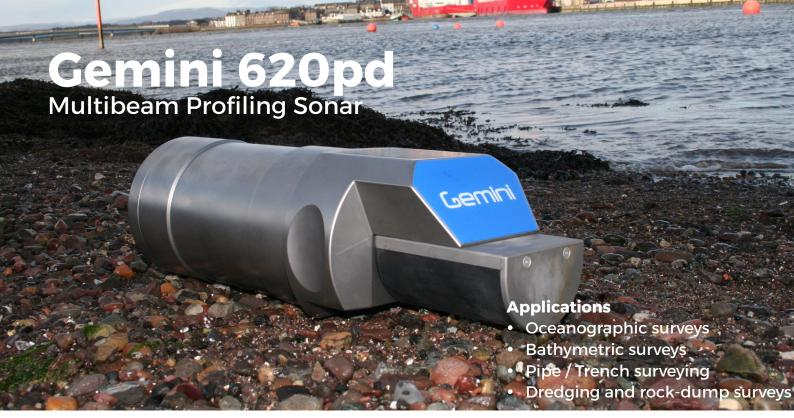
The Gemini 620pd benefits from the latest technological advances in signal processing. These allow the 620pd to produce high performance bathymetry data, which can be output to industry recognized survey packages for processing. Designed for Remotely Operated Vehicle (ROV) mounting, the Gemini 620pd is manufactured in titanium and rated to an operational depth of 4000m.
