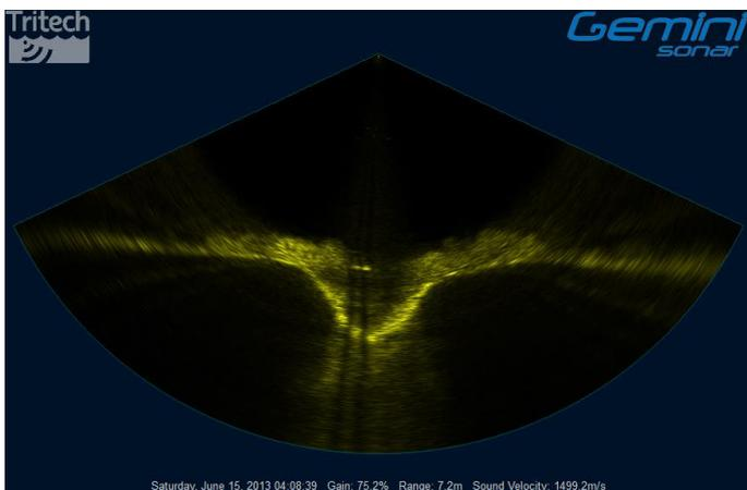
Trittech's Gemini NBI Image of an excavation operation showing the clear visibility of a cable being trenched (image courtesy of Reef Subsea Dredging & Excavation).
