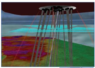
(Top) Illustration of Tritech RAMS deployed through a fixed internal turret on an FPSO.
