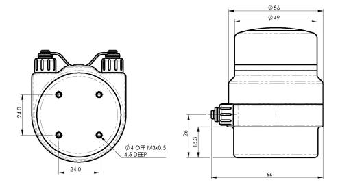
Not to scale. Measurements in mm.
