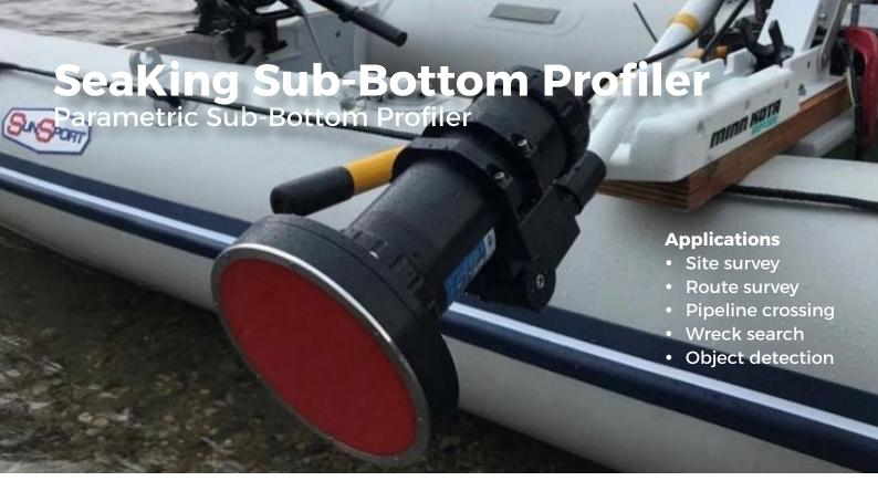
The specially designed transducer enables the echosounder to emit very low frequencies whilst minimising the size of the overall unit. Producing a 20kHz pulse, the system is capable of penetrating the seabed and highlighting structural differences that are hidden from view to conventional echosounders.
