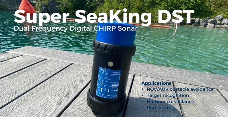
The V7 Super SeaKing DST mechanical scanning sonar now offers enhanced performance and the option of Ethernet communication for high speed scanning over short ranges. Retaining dual frequency capability, the Super SeaKing DST can achieve 300m range at 325kHz, with increased image intensity and with improved mid-water target discrimination capability at 650kHz.
