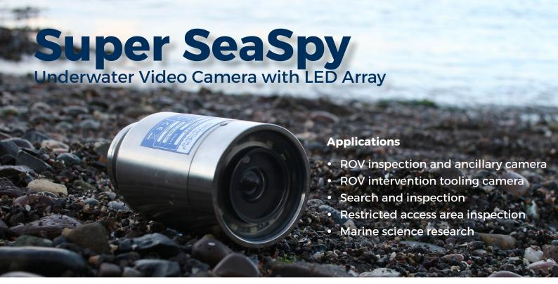
An integrated array of high power LEDs ensures the camera always has light to operate. The Super SeaSpy is also fitted with an Ivanoff corrected lens system that optimises the picture quality by reducing radial distortion and reducing chromatic aberration. An additional integral video line driver can be fitted to compensate for attenuation of the signal when used through longer cables.
