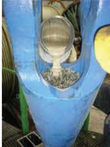
FIGURE 8.53 Spelter socket with wire splayed and technician pouring in epoxy binder.
