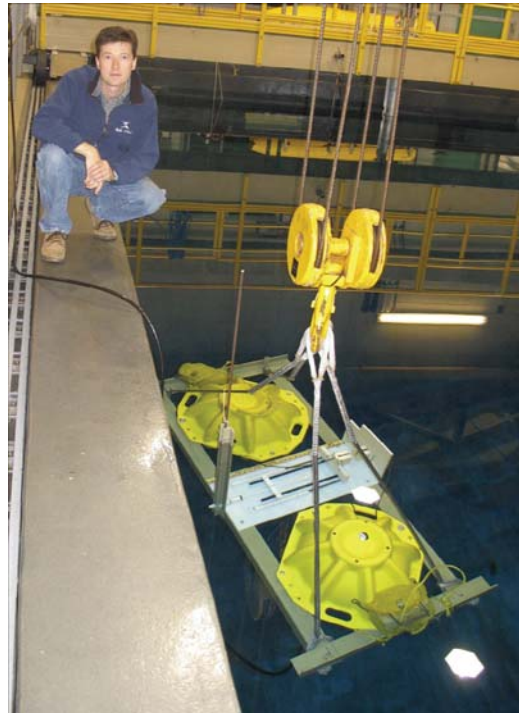
FIGURE 8.38 MBARI tests bluetooth between glass spheres.
